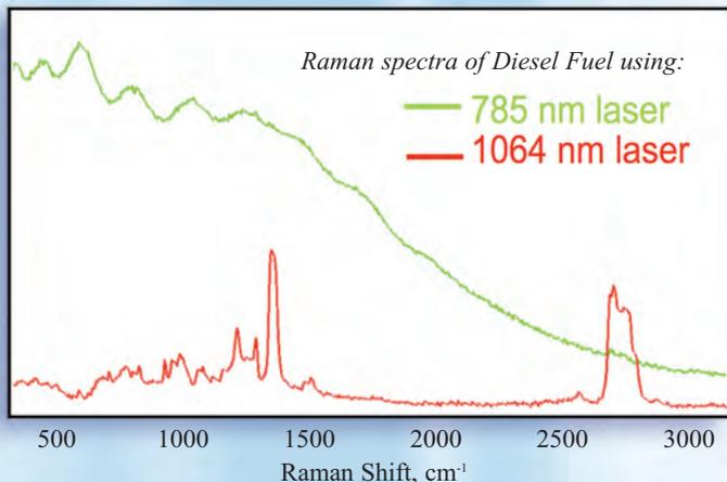
Excitation with a 785 nm laser produces featureless fluorescence in this diesel fuel, while excitation with RTA's 1064 nm laser produces a quantifiable Raman spectrum.
