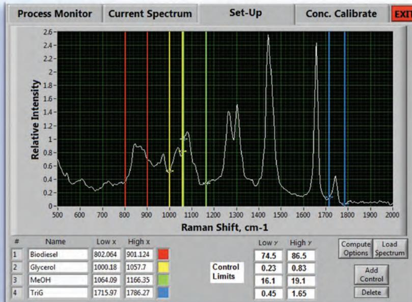
Raman spectrum representative of biodiesel production. Colored lines indicate spectral regions used to monitor biodiesel, glycerol, methanol and triglycerides for a batch reactor.
